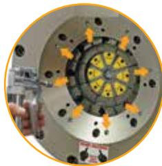
Easy grease maintenance through the 8 lubrication fittings.
