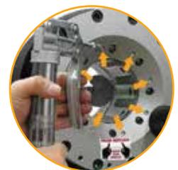
Easy grease maintenance through the 8 lubrication fittings.
