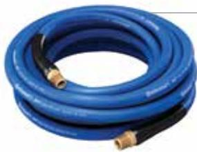
A hybrid thermoplastic hose that provides durability and flexibility, is lightweight and has a low drag resistance. F5™ is non-marking, oil resistant and performs well under cold temperatures to -40°F (-40°C) and temperatures as high as 158°F (70°C). This 300 psi hose is designed for a variety of pneumatic applications in industries such as construction and manufacturing.
