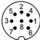
Pin assignment of S32 (view of connector pins of transducer), 8-pin M16 circular plug
