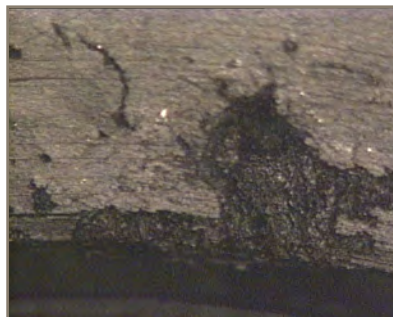
Pitting on filter end-cap
