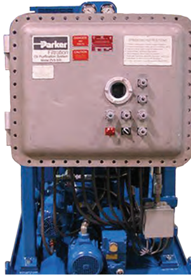
NEMA 7 Explosion Proof
